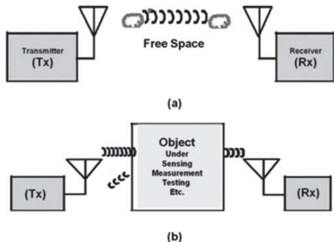
Figure 2. Radio-wave system (a) communication and (b) measurement.
