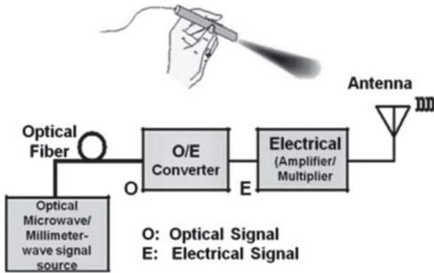
Figure 3. Photonic-assisted MW/MMW Transmitter.
