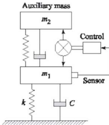
Figure 6. Schematic Diagram for Hybrid Control System.
