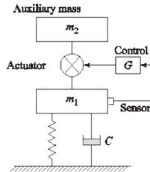
Figure 4. Schematic Diagrams for Active Control System.
