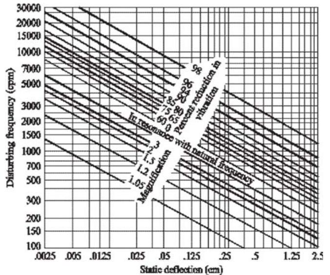
Figure 9. Isolation Efficiency of Resiliently Mounted System.
