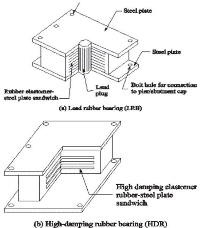
Figure 13. Seismic Isolation Devices.
