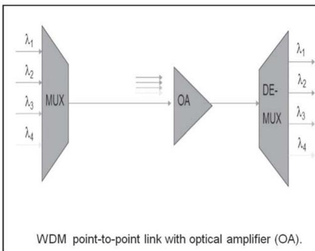
Figure 4. WDM-Optical Amplifier.
