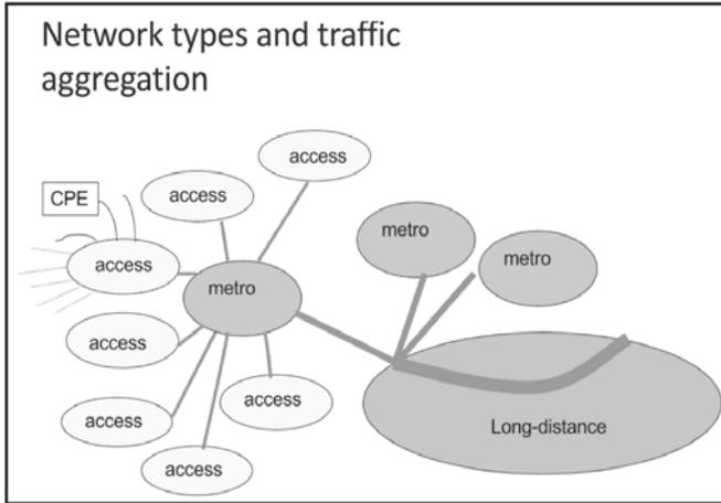
Figure 7. Three types of networks: Traffic Aggregation.
