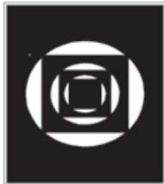
Figure 4. Crown antenna structure after third iteration.
