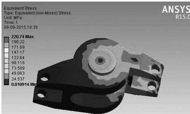
Figure 4. Vonmises stress (steel)
