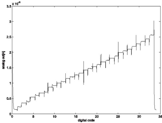
Figure 8. Simulation of 5-bit DAC.
