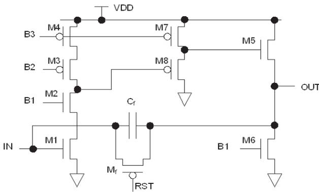
Figure 2. Circuit diagram for pre-amplifier.
