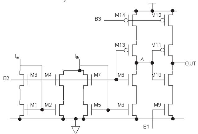
Figure 4. Schematic diagram of comparator.
