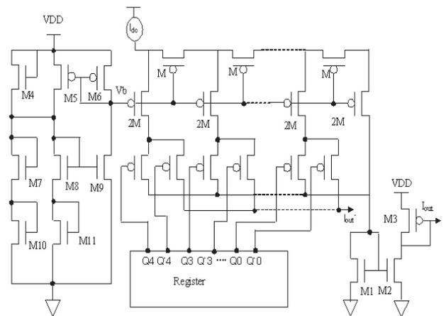
Figure 7. Block schematic of the 5-bit current DAC.
