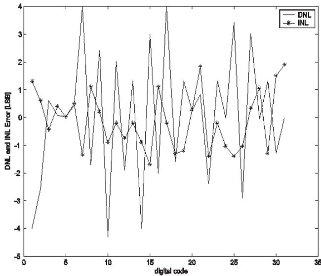
Figure 9. Differential and integral nonlinearity errors.
