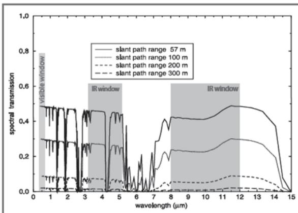
Figure 3. Spectral Transmission for CAT III Fog.
