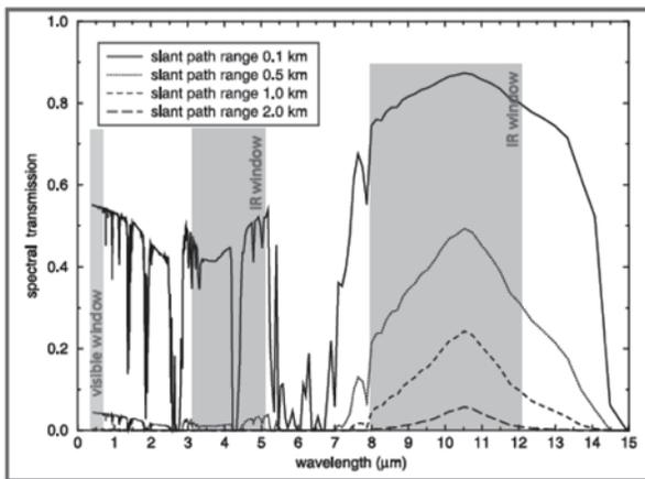
Figure 2. Spectral Transmission for CAT II Fog.
