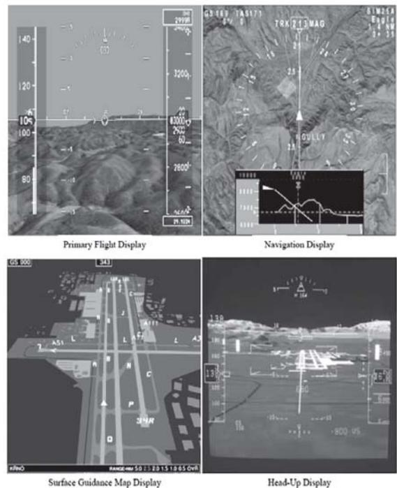
Figure 4. Examples of Synthetic Vision System Displays.
