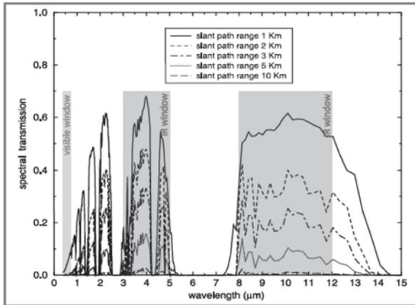
Figure 1. Spectral Transmission for CAT I Fog.
