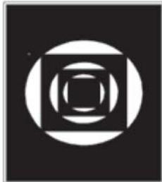
Figure 4. Crown antenna structure after third iteration.
