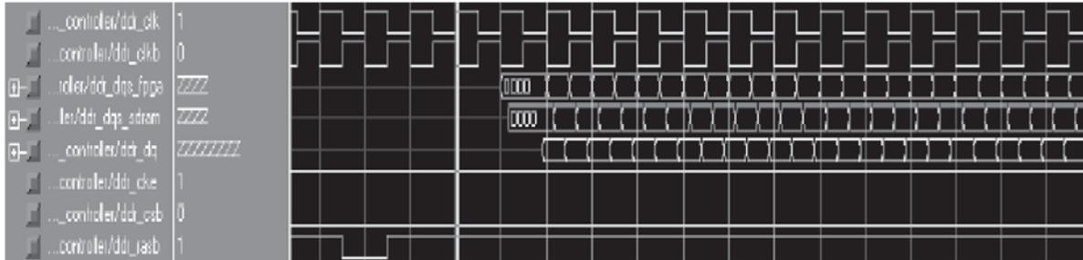
Figure 7. Write of burst length 8.
