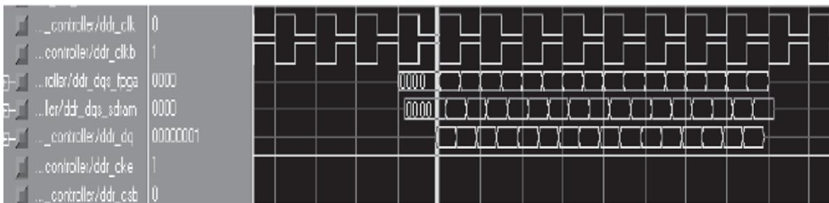
Figure 6. Write of burst length 4.
